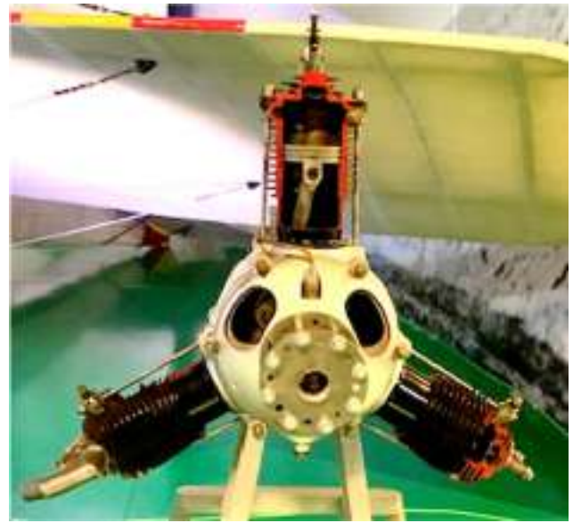
Figure 3: and here we can see the Museum's 35 HP Anzani with “Y” cylinders at 120°.
