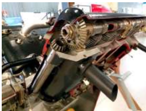
Figure 1: This image shows the camshaft and the bevel gears connecting to the drive shaft from the crankshaft.
