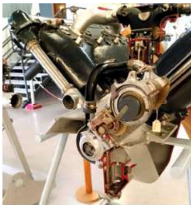
Figure 3: in this image you can see the water and oil pumps, as well as an installed magneto and the connection for the other magneto. The cooling water inlet tube (black) starts from the water pump to both blocks.
