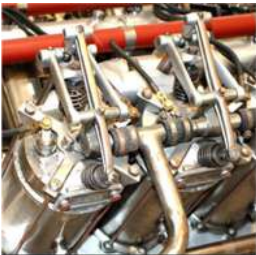
Figure 2: Detail of the upper cylinder fastenings and the set of rocker arms and valves.
