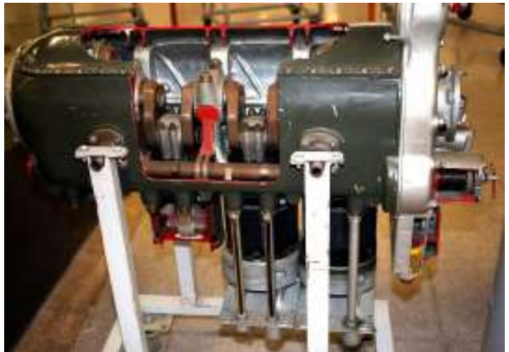
Figure 1: Cutaway engine on display showing crankshaft and connecting rod joints.
