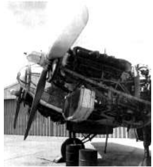
Figure 5: Merlin 500-29 engine installed in a CASA 2111 aircraft.
