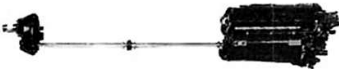
Figure 5: Side view of the Model E V-1710 showing the two 4-foot-long, 2.5-inch-diameter extension shafts terminating in the propeller reduction gearbox. Fuselage flex and misalignment are controlled by internally splined flexible couplings.
