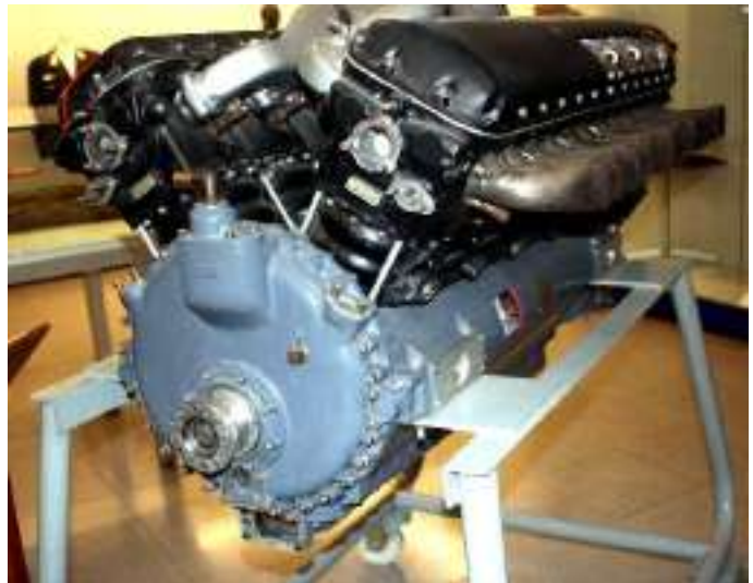
Figure 1: This image shows the front flange, crankshaft extension, to which the extension shaft for the propeller is bolted.
