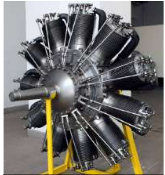
Siemens Halske Sh III 11-cylinder counter-rotary.
