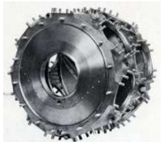
Main crankcase composed of four casings joined by rivets.
